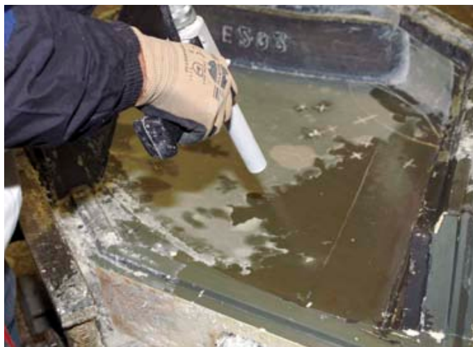
Thanks to the gentle Ascojet dry ice blasting, tool wear has been significantly reduced.
