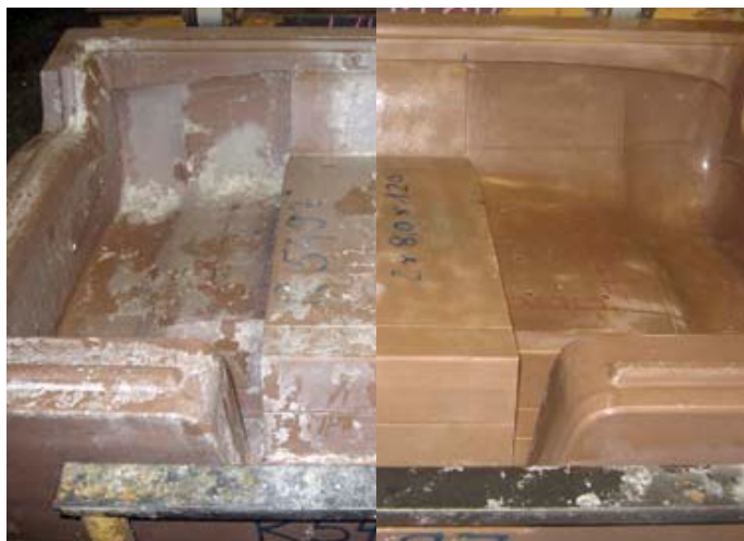
PU foaming tools before and after cleaning with dry ice.
